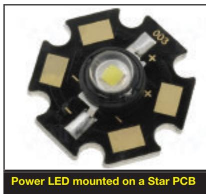
Power LED mounted on a Star PCB
